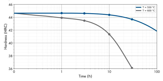
VH13 | VH13SI $^{\circ}$  resistance to softening. After 30 h, hardness decreases only 1,0 HRC at 550  $^{\circ}$ C and 9,0 HRC at 600  $^{\circ}$ C.
