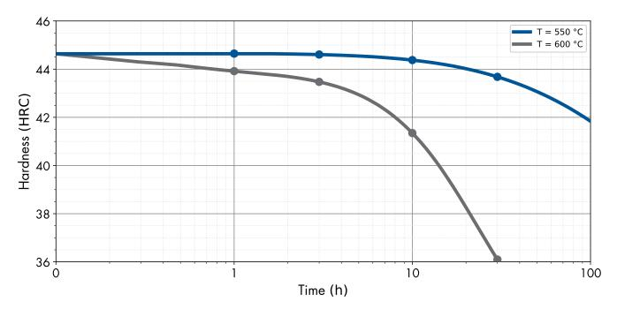
$$V2344^{\circ}$$  resistance to softening. After 30 h, hardness decreases only 1,0 HRC at 550 °C and 9,0 HRC at 600 °C.
